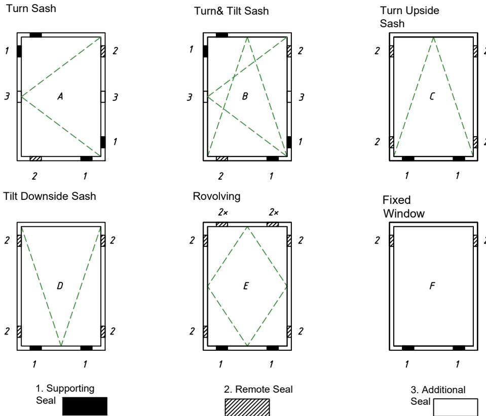
Supporting Seal-in Case Of Revolving Sash
